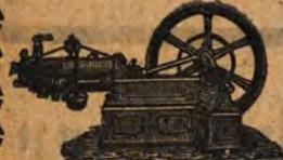
Gasmotore eigener Construction,
