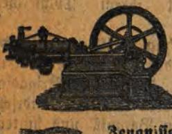
Gasmotore eigener Construction,
